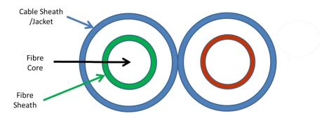
Typical Cable Construction – Multi-Core Cable
